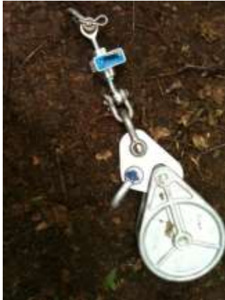
Figure 3 (left) the wireless dynamometer attached to the end-block, (right) rigging the end-block at 6 m.
