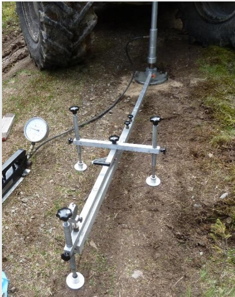
measuring of "EV2" [ MPa ], using "Static load plate test" device
